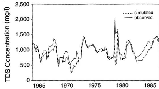
Fig. 6. Simulated and observed TDS concentrations at the Whitney gauge.
