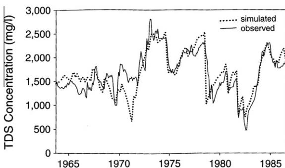
Fig. 5. Simulated and observed TDS concentrations at the Graford gauge.
