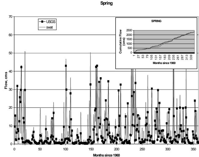
**Figure 2c.** The SWT predicted and USGS (measured flows on the Spring (12040102) sub-basin of San Jacinto. Inset is cumulative flow.
