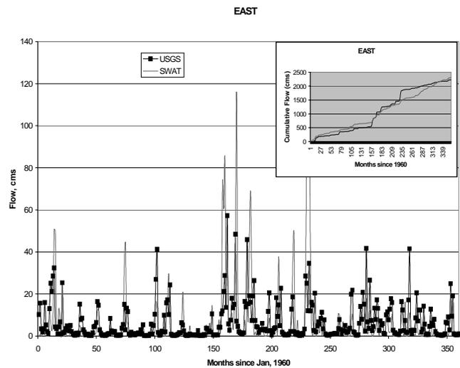
Figure 2a. Monthly SWAT and U.S. Geological Survey (USGS) measured flows after calibration for the East Fork (12040103). Inset is comparison of cumulative flows.
