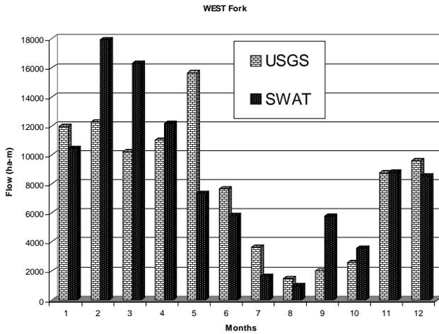
**Figure 2b.** Bar chart of averaged flows (in units of hectare-meters/month) of SWAT and USGS (id=8069500) flows based on monthlies during 1929 to 1954 after calibration of SWAT parameters on the West Fork of San Jacinto (12040101).
