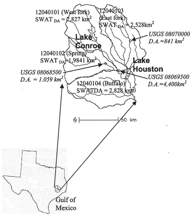
**Figure 1.** San Jacinto river basin; SWAT<sub>DA</sub> is the drainage area estimated by the Soil and Water Assessment Tool (SWAT) model using GIS data.
